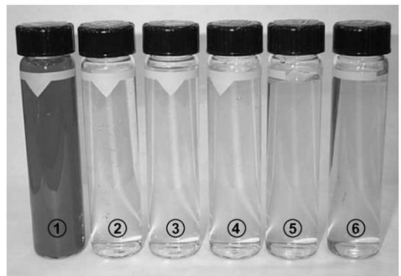
Fig. 9. Comparison of purified samples. No. 1: original slurry. Nos. 2–6: the flow rate is 0.1, 0.5, 1.0, 2.0 and 3.0 l/min, respectively.
