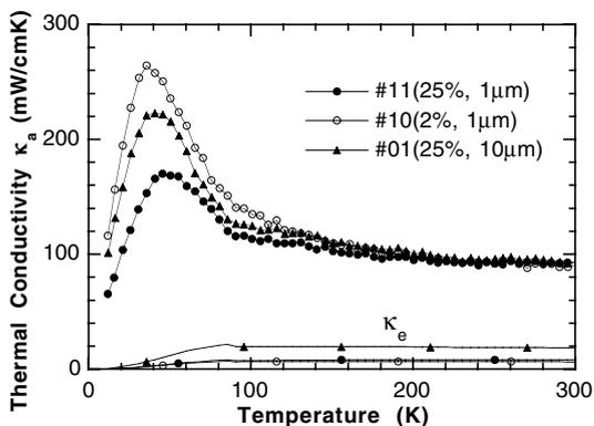
Fig. 3. The temperature dependence of the  $a$ -axis thermal conductivity  $\kappa_a(T)$  under the zero field. The estimated electronic thermal conductivity  $\kappa_e$  is also shown.
