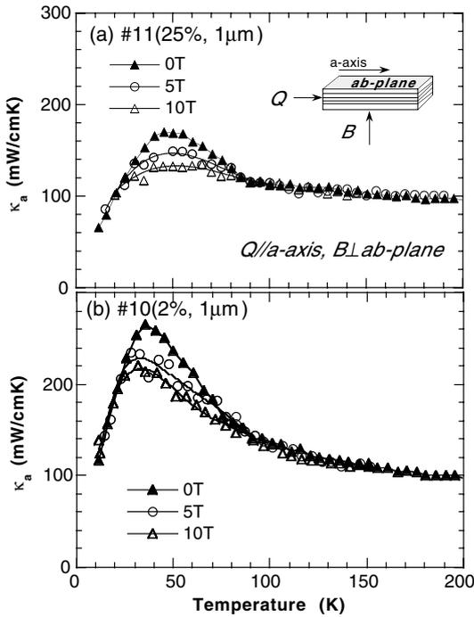
Fig. 4. Magnetic field dependence of  $\kappa_a(T)$  for the (a) #11(25%, 1  $\mu\text{m}$ ) and (b) #10(2%, 1  $\mu\text{m}$ ) specimens.
