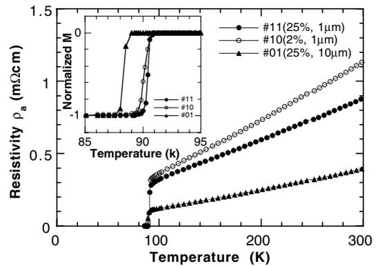
Fig. 1. The  $a$ -axis electrical resistivity  $\rho_a$  of the three specimens (#11(25%, 1  $\mu\text{m}$ ), #10(2%, 1  $\mu\text{m}$ ) and #01(25%, 10  $\mu\text{m}$ )) as a function of temperature  $T$ . The normalized magnetization  $M$  is also shown in the inset.
