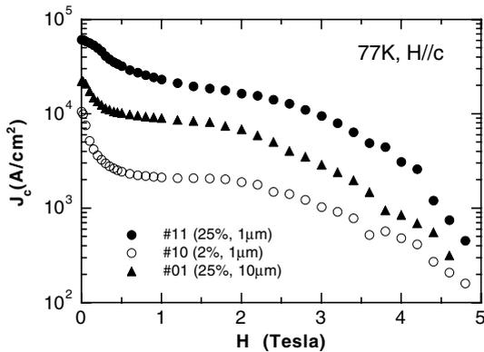
Fig. 2. The magnetic field dependence of the critical current density  $J_c$  at 77 K for three specimens.
