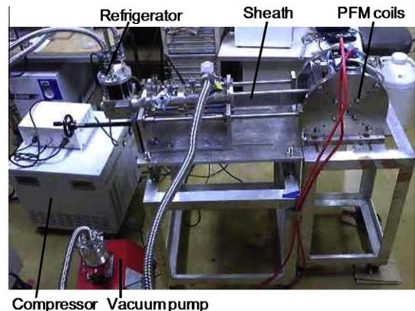
Fig. 2. Strong field generator containing five-aligned bulk magnets in the sheath and magnetizing coil to activate them.
