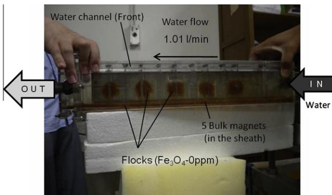
Fig. 8. View of the magnetic separation experiment for the flocks with no magnetite powder addition with a flowing rate of 1.01 l/min.
