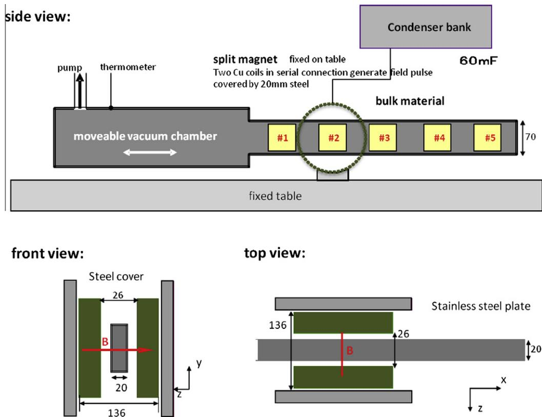
Fig. 3. Schematic illustrations of bulk magnet system and magnetizing apparatus to apply pulsed fields.
