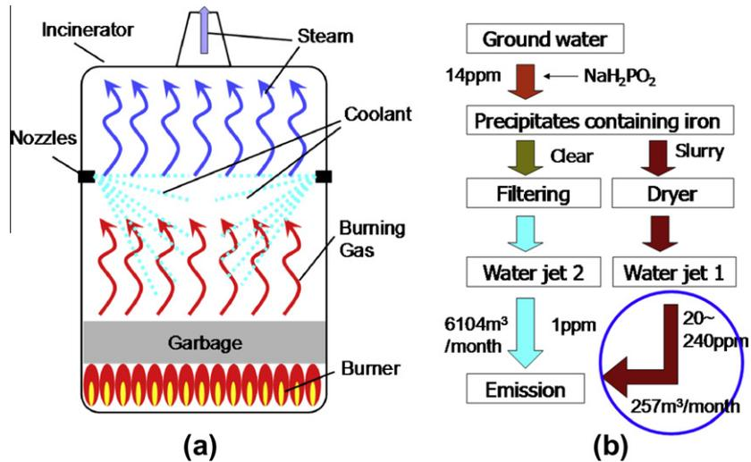
Fig. 1. Schematic illustration of waste material disposal furnace (a) and water purification process of groundwater (b).
