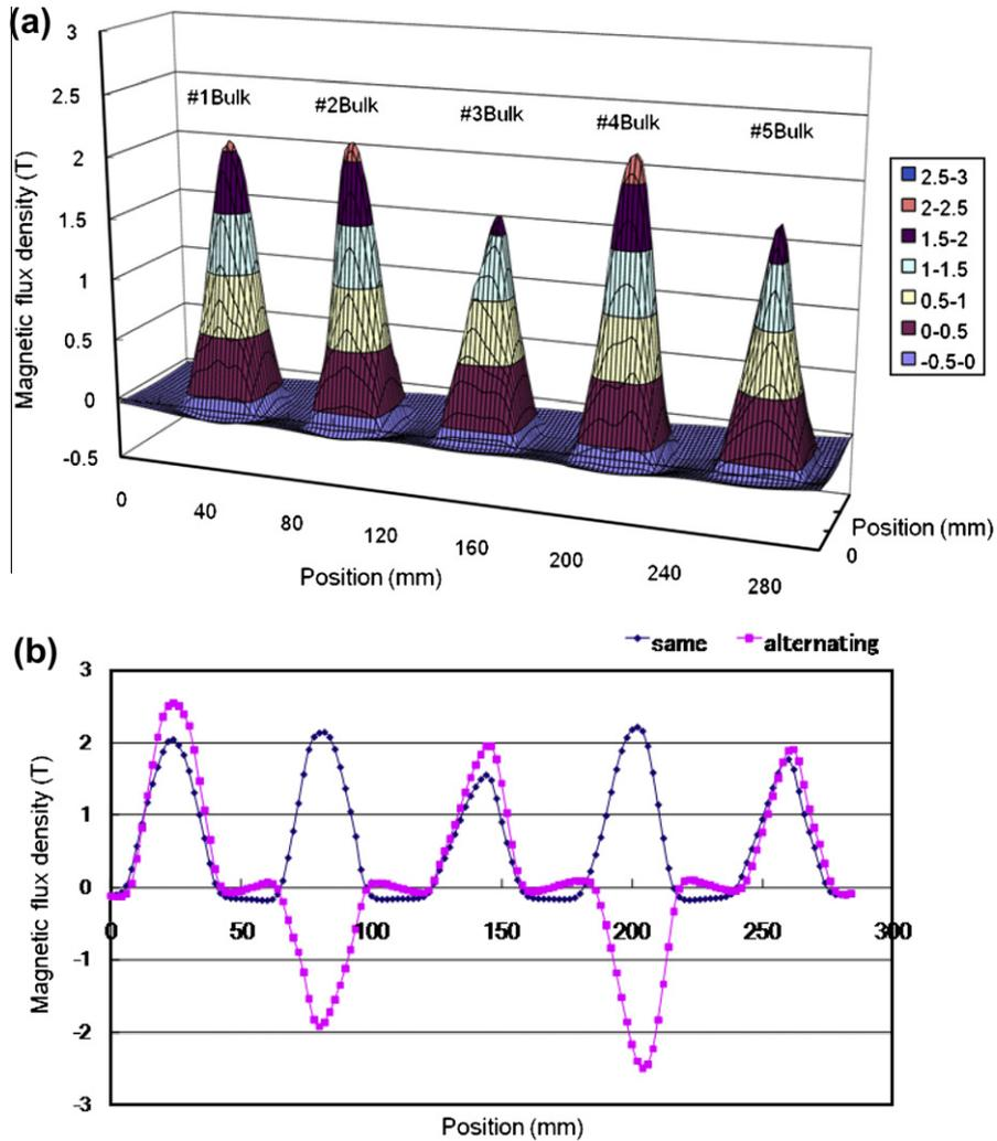
Fig. 5. Three dimensional distribution of trapped magnetic field on the sheath surface (a), and cross sectional distribution with same and alternating magnetic pole arrangement (b).
