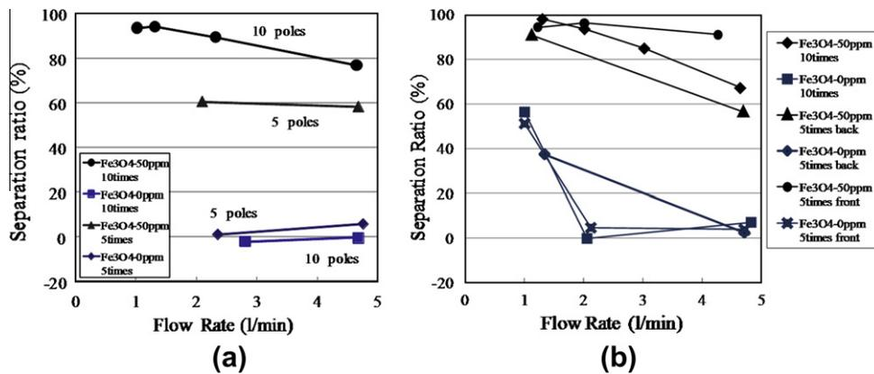
Fig. 7. Flow rate dependence of separation ratio for same (a) and alternating (b) magnetic pole arrangement.
