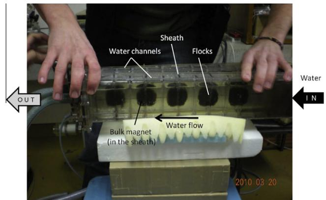
Fig. 6. Photo of the experiment by open gradient magnetic separation technique.
