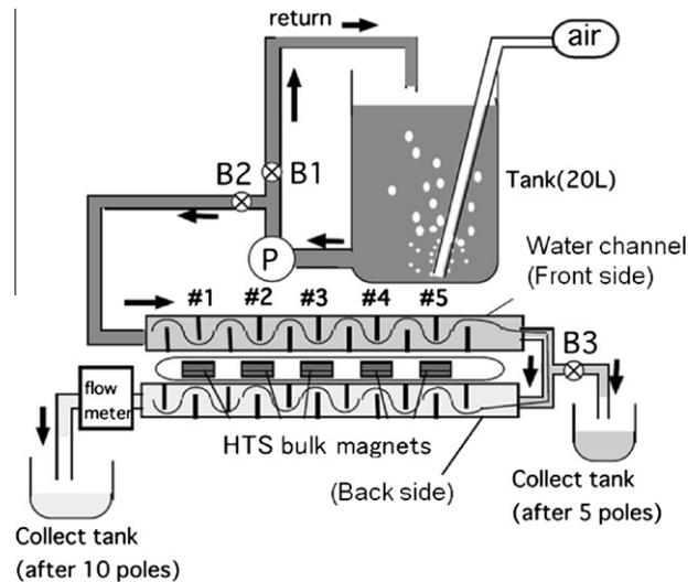
Fig. 4. Schematic structure of magnetic separation experiment with use of a couple of water channels which are attached beside the multi-pole magnetic sheath.
