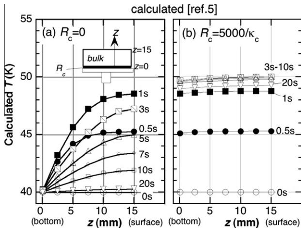
**Fig. 1.** Time dependence of calculated temperature changes  $T(z, t)$  as a function of the distance  $z$  from the bottom of the YBCO bulk after the pulse field application, which were shown in Ref. [5]: (a) is for the ideal but unrealistic case with the contact thermal resistance of  $R_c = 0$  and (b) is for the optimum case.
