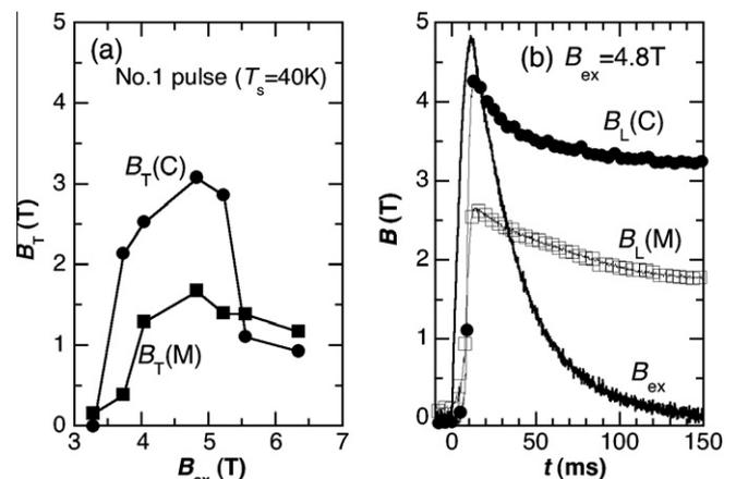
**Fig. 3.** (a) The trapped field  $B_T$  as a function of applied field  $B_{ex}$  at the center (C) and the middle (M) positions on the bulk. (b) The time evolution of the applied field  $B_{ex}(t)$  and local fields ( $B_L(C)(t)$  and  $B_L(M)(t)$ ) after applying pulsed field of  $B_{ex} = 4.8$  T at  $T_s = 40$  K.
