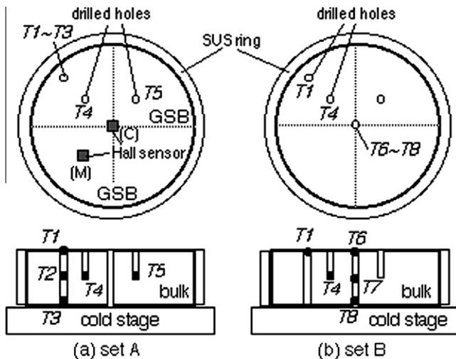
**Fig. 2.** The measuring position of temperatures  $T(t)$  and magnetic fields  $B_L(t)$  for (a) “set A” and (b) “set B”.
