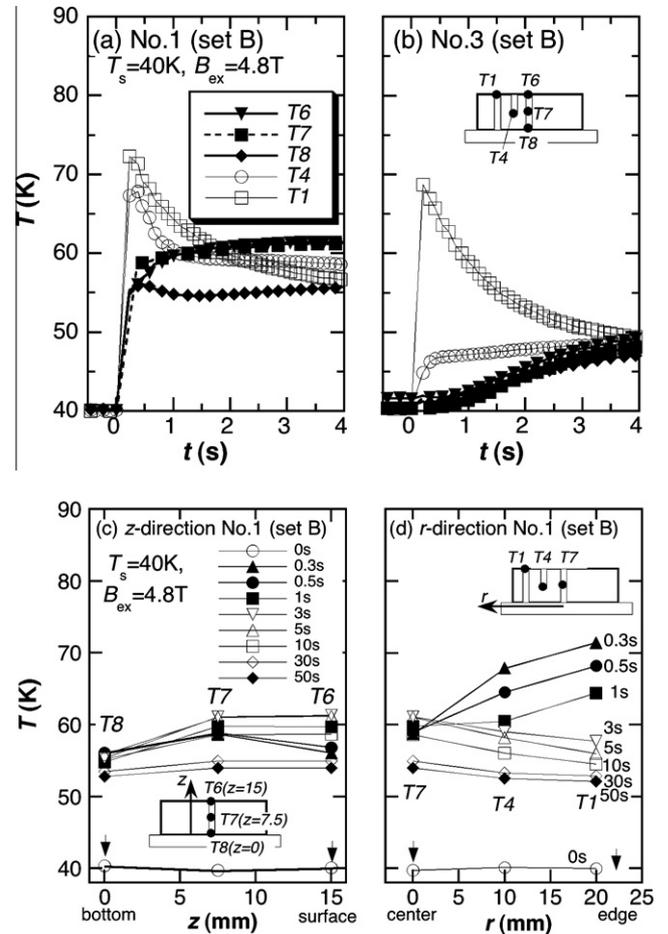
**Fig. 5.** Time evolution of temperatures ( $T1(t)$ ,  $T4(t)$ ,  $T6(t)$ – $T8(t)$ ) for “set B” after applying pulsed field of  $B_{ex} = 4.8$  T of the (a) No. 1 and (b) No. 3 pulse. (c) The temperature changes for the No. 1 pulse, as a function of the distance  $z$ . (d) The temperature changes for the No. 1 pulse as a function of the distance  $r$ .
