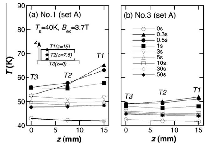
**Fig. 6.** The time evolution of the temperatures  $T(z, t)$  as a function of the distance  $z$  in “set A”, after applying the (a) No. 1 and (b) No. 3 pulses of  $B_{ex} = 3.7$  T at  $T_s = 40$  K.
