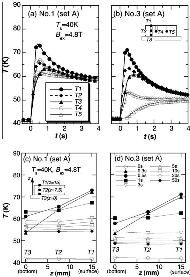
**Fig. 4.** Time evolution of temperatures ( $T1(t)$ – $T5(t)$ ) for “set A” after applying pulsed field of  $B_{ex} = 4.8$  T of the (a) No. 1 and (b) No. 3 pulse. The temperature changes for the (c) No. 1 and (d) No. 3 pulse, as a function of the distance  $z$  from the bottom of the bulk, which were re-plotted using (a) and (b), respectively.
