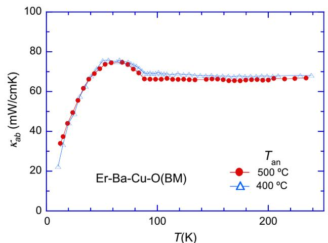
Fig. 2. The temperature dependence of the *ab*-plane thermal conductivity of Er-Ba-Cu-O bulk superconductors for  $T_{\text{an}} = 400^\circ\text{C}$  and  $500^\circ\text{C}$ .
