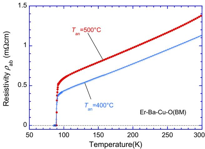
**Fig. 3.** The temperature dependence of the  $ab$ -plane electrical resistivity,  $\rho_{ab}(T)$ , of Er–Ba–Cu–O bulk superconductors for  $T_{an} = 400^\circ\text{C}$  and  $500^\circ\text{C}$ .
