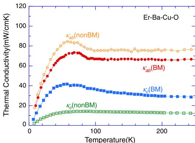
Fig. 1. The temperature dependence of the *ab*-plane and *c*-axis thermal conductivity,  $\kappa_{ab}(T)$  and  $\kappa_c(T)$ , for Er-Ba-Cu-O bulk superconductors ( $T_{\text{an}} = 450^\circ\text{C}$ ). The closed and open symbols, respectively, represent the Er-Ba-Cu-O bulk with the ball-milled (BM) and nonBM Er211.
