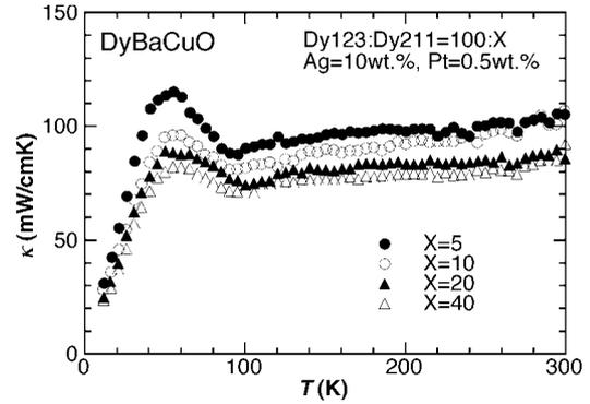
**Figure 2.** The *ab*-plane thermal conductivity  $\kappa(T)$  for the DyBaCuO bulk for various Dy211 contents  $X$ .
