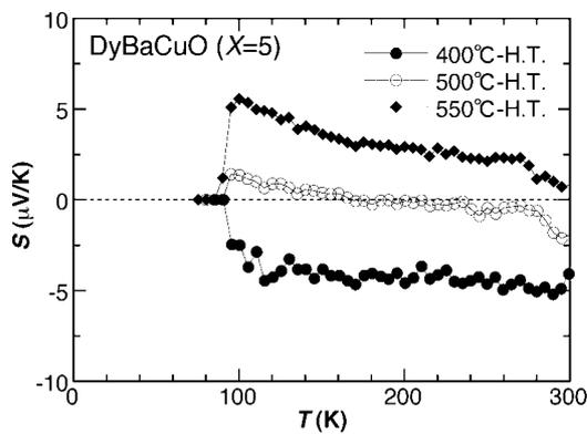
**Figure 4.** The temperature dependence of the  $S(T)$  for the  $X = 5$  samples with different heat treatment temperatures  $T_{HT}$ .
