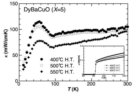
**Figure 5.**  $\kappa(T)$  for the  $X = 5$  samples with different  $T_{HT}$ . The inset shows the resistivity  $\rho(T)$  for the same samples.
