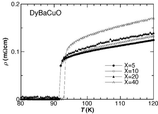
**Figure 1.** The temperature dependence of the *ab*-plane electrical resistivity  $\rho(T)$  for the DyBaCuO bulk for various Dy211 contents  $X$ .
