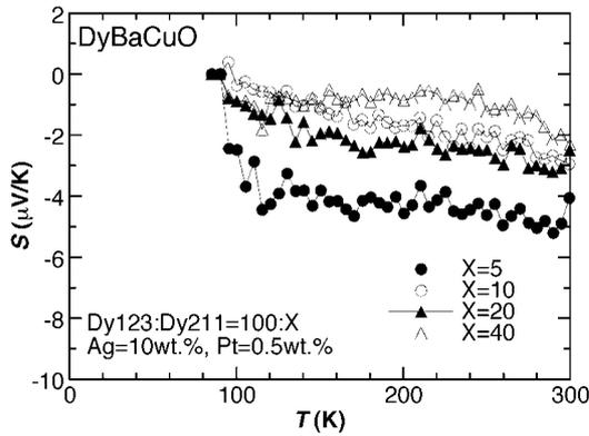
**Figure 3.** The *ab*-plane thermoelectric power  $S(T)$  for the DyBaCuO bulk for various Dy211 contents  $X$ .
