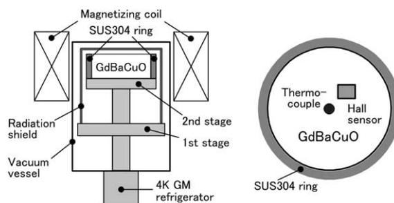
Fig. 1. Experimental equipment.
