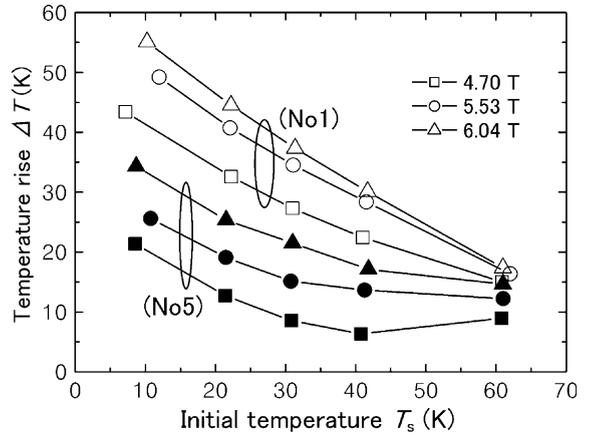
Fig. 3. The initial temperature  $T_s$  dependence of temperature rise  $\Delta T$  after applying the first (No1) and the fifth (No5) pulsed field for various applied fields  $B_{ex}$ .
