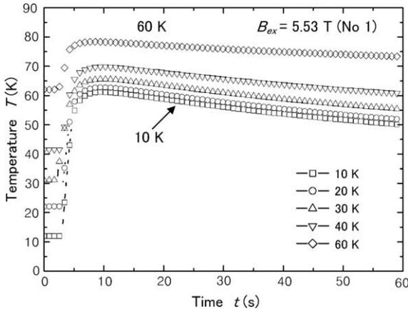
Fig. 2. The time responses of temperature  $T(t)$  at the initial temperatures  $T_s$  ranging from 10 to 60 K after applying the first pulsed field of 5.53 T.
