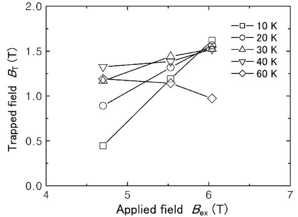
Fig. 5. The  $B_{ex}$  dependence of the trapped field  $B_T$  for each  $T_s$ .
