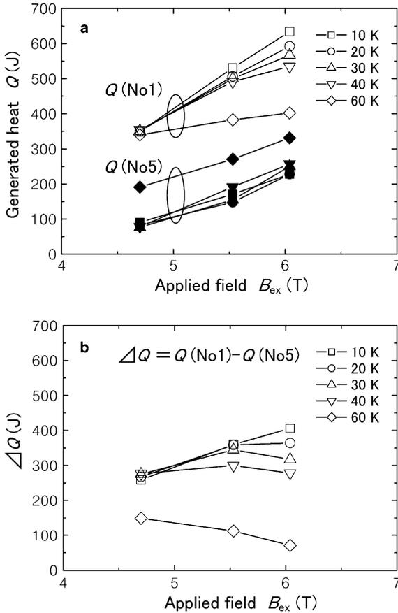
Fig. 4. (a) A generated heat  $Q(\text{No1})$  and  $Q(\text{No5})$ , and (b)  $\Delta Q = Q(\text{No1}) - Q(\text{No5})$  at  $T_s = 10$ –60 K as a function of  $B_{ex}$ .
