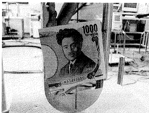
Fig. 17 The magnetic attraction of Japanese 1000 yen bill on the surface of the bulk magnet.
